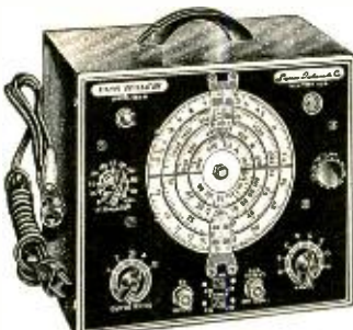
• Tubes used: 1-6BE6 as R. F. Oscillator, mixer and amplifier, 1-6BE6 as Audio Oscillator, 1-6HG as Power Rectifier.
